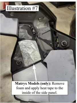
25. Check the clearance between the side panel and the exhaust silencer. Due to chassis variation, some sleds will need the foam removed from the top inside of right hand side panel and install provided heat tape and others will not (see illustration #15).
