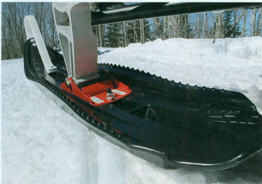
A change in ride height caused by skis will affect how a rear suspension functions, and the front bumper on our Adventure ended up three-sixteenths of an inch closer to the ground with the SLP skis installed. Fortunately, that was not enough to cause a change in suspension and chassis performance or feel.
